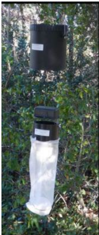
Photograph 16. View of a CO 2 trap, which lures many species of mosquitoes with dry ice, which mimics the smell of an exhaling animal. These traps are set overnight at the margins of vegetation transitions. (Source: MVDSBC 2026 )
